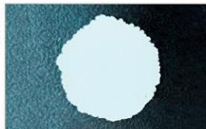
Heat at 200°C for 15 minutes, the sealer remains stable in its properties. ▶
