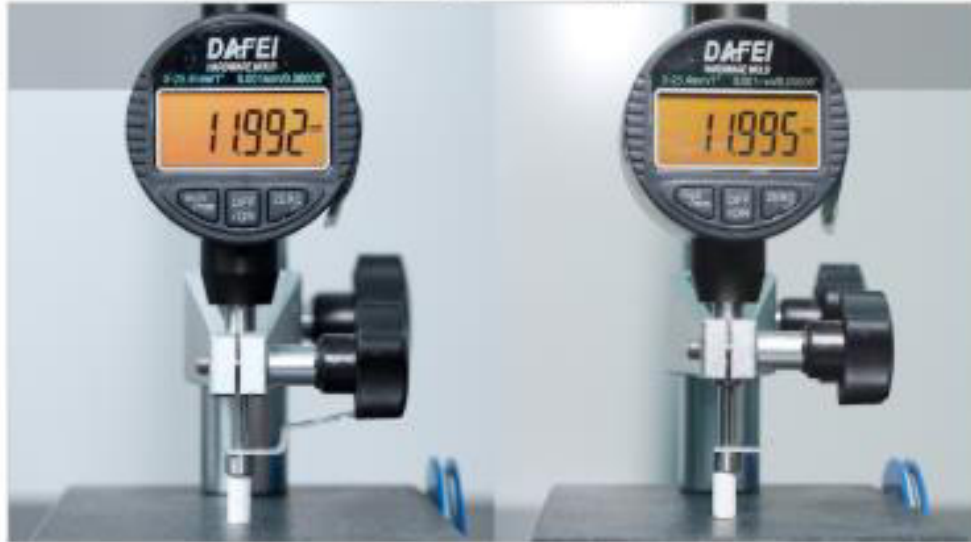
Tests showing the expansion rate of 0.025%.
