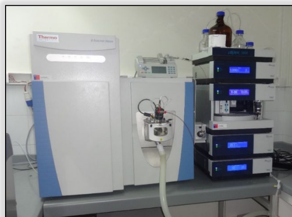
Figura 18. Ultra High Performance Liquid Chromatography- Electrospray ionization- Quadrupole-Orbitrap-Mass Spectrometry (UHPLC-ESI-Q-Orbitrap-MS/MS)
