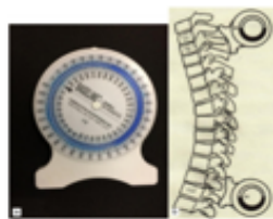
Figure 1. (a) The gravity-dependent analog bubble inclinometer and (b) an illustration of the application of the gravity-dependent inclinometer.
